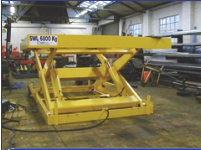
Scissor lift manufactured in our fabrication shop before truck-dock assembly.
